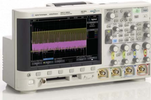
The 1M-waveform/sec update rate, optional built-in waveform generator, and moderate price are among the features that distinguish the MSO-X 3054A 500-MHz-analog-bandwidth mixed-signal scope. With the optional double-depth memory and two analog channels in use, the scope acquires 4M-sample records at 4G samples/sec/channel.
